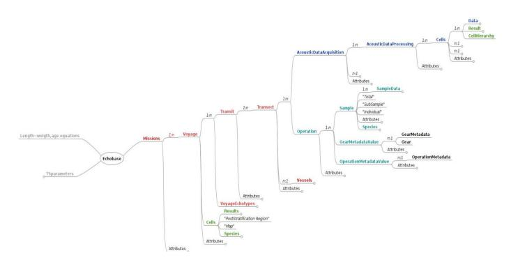
Figure 3. EchoBase data model. Cruise metadata branch in red, acoustic branch in blue, fishing (operation) branch in teal, results branches in green, reference relationships in grey.
