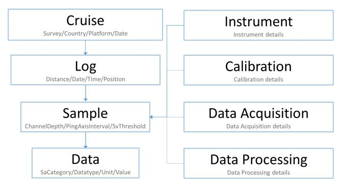
Figure 6. Hierarchical view of the Acoustic data model.
